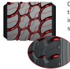
Cap shaped tie bars allow tires to self clean for improved traction and stability.
